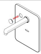
3. Turn the Disinfection Key 180° to remove it and install the key cover.
