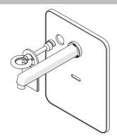
2. Hang the warning tag plate on the Disinfection Key, insert the Disinfection Key and turn it 180° (direction not important). Place the warning tag in the keys' groove. Activate "Continuous run" Function (See section 7.2 SENSOR SETTING INSTRUCTIONS).
